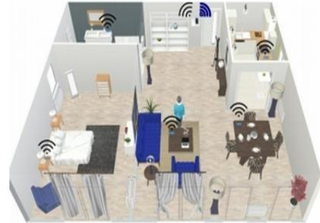
Fig 1: SensePods for smart homes forming an ad-hoc ZigBee network
